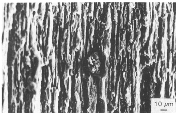
Figure 9 Scanning electron micrograph of tensile fracture surface of alloy 8090 showing typical mixed mode of failure.
